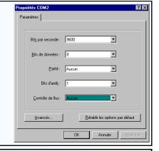
6 The PC is now in terminal mode, connect it to the device by plugging the RS232 cable.
